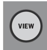
Each major section of the console's top panel has a button called VIEW. Pressing one of these will switch the Main Display to a dedicated screen for the section whose VIEW button was pressed. The Main Display will often have additional parameters, options or information that is not accessible from the top panel alone.
