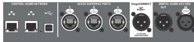
A pair of Ethernet ports allow a network to be set up via router for wired or wireless control using one of the control apps for PC, phone or tablet. A USB port allows bidirectional 48-channel transmission as well as firmware updates and data exchange. An ASIO driver can be downloaded from [behringer.com](http://behringer.com).
